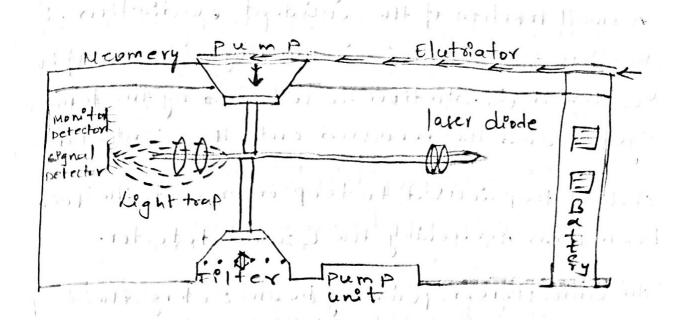
A small pump Draws the Dust-laden air at the orate of 0.625 liters/non through the parllel plate Elutoactors to Remove the Non-Respurable Dust, though a light beam and then filter so that the Dust an be and for further analysis. The use of the filter also Enables instrument Calibration.
